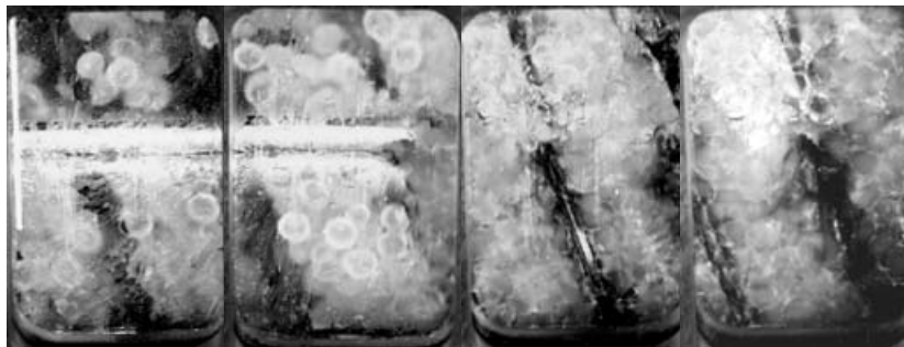
Figure 2a. 27Kg/Hr (60PPH)/60RPM Melting Sequence Visualization: Solid Conveying and Compaction Region
